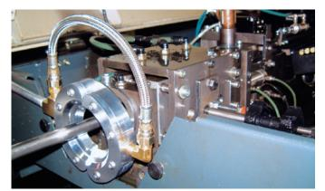
The Super Air Wipe eliminates the possibility of smoke during machining by wiping hydraulic oil from the bar stock as it enters the chuck.
