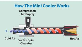
The Mini Cooler incorporates a vortex tube to convert a small amount of compressed air into two low pressure streams, one moving within the other in opposite directions (see page 200). The two airstreams exchange heat, producing cold air from one end of the tube and hot air from the other. A flexible hose directs the cold airstream at the surface to be cooled.
