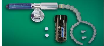
Model 3925 Adjustable Spot Cooler System includes the Adjustable Spot Cooler, dual point hose kit with cone and fan nozzles, swivel magnetic base, filter separator, 15 and 30 SCFM (425 and 850 SLPM) generators. (25 SCFM/708 SLPM generator installed.)
