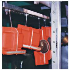
A Model 110018 18" (457mm) Super Air Knife cools molded plastic following dip molding.
