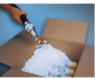
A Model 130125 1-1/4" (32mm) Light Duty Line Vac can fill or empty the packing peanuts from shipping cartons.
