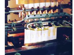
A Model 2012 12" (305mm) Standard Air Knife opens mustard packets prior to fill.
