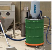
Sand that covers the floor around a sand blaster is quickly vacuumed into the drum using the rugged floor tool.
