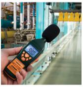
The Sound Level Meter identifies a potential source of hearing loss.
