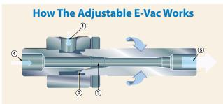
Compressed air flows through the inlet (1), then through an adjustable annular nozzle (2). As the airstream enters the vacuum flow, it expands and increases in velocity (3). A vacuum flow is induced, creating suction (4). The airflow that is drawn through the vacuum inlet mixes with the primary airstream, then exhausts on the opposite end (5).
