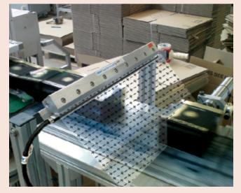
**The Problem:** A manufacturer of perfumes and fragrances had a problem with the packaging of their fine perfumes. The conveyor belt used to transport the boxes to the cellophane sealer rubbed against the box surface and induced a sizable static electricity charge on it that made it a "dust magnet". The cardboard dust and particulates
