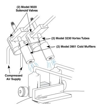
**The Problem:** Air conditioner parts assembled on an automatic brazing machine must be cooled to handling temperature prior to removal. The machine was capable of brazing up to four hundred pieces per hour. However, the time required for the parts to cool severely limited the production rate. Water cooling was unacceptable from the standpoint of both housekeeping and part contamination.
