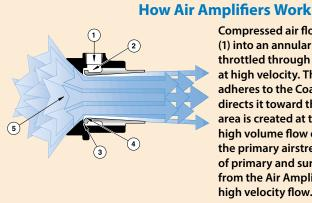
Compressed air flows through the air inlet (1) into an annular chamber (2). It is then throttled through a small ring nozzle (3) at high velocity. This primary airstream adheres to the Coanda profile (4), which directs it toward the outlet. A low pressure area is created at the center (5), inducing a high volume flow of surrounding air into the primary airstream. The combined flow of primary and surrounding air exhausts from the Air Amplifier in a high volume, high velocity flow.
