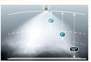
1/8 NPT Internal Mix Flat Fan atomizing nozzles can apply a light or heavy film coat to products moving on a conveyor.
