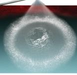
The precision machining of the HollowStream nozzle produces a controlled spray angle in this rinsing operation.
