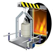
The timer was set to "on/off delay". The sensor was mounted at the oven exit (1 minute away from the blowoff station). When the sensor detected a tank, the timer turned the air on for one minute, just as the next tank reached the blowoff station.
