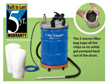
The Chip Trapper includes the pump assembly with directional flow valve, a 30, 55 or 110 gallon drum, 10' (3m) chemical resistant hose, 20' (6.1m) compressed air hose, aluminum chip wand, (2) reusable 5 micron filter bags and drum dolly.
