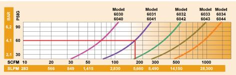
Total Output Flow with .002" (0.05mm) gap setting. Excludes downstream entrainment.
