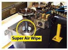
The flanged end of an axle is lifted through a Super Air Wipe to blow off chips after machining.
