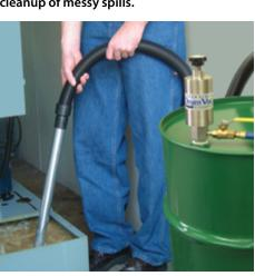
Reversible Drum Vacs are designed to fit the 3/4 NPT bung of any closed top drum. This Model 6196-30 30 gallon system empties the coolant sump of a CNC.
