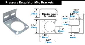
This optional mounting bracket fits Models 9008, 9033 and 9009 Pressure Regulators and includes a locking ring.
