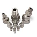
EXAIR's Swivel Fittings make it easy to adjust the position of the Air Nozzles, Air Jets, and Air Amplifiers. Swivel Fittings permit a movement of 25 degrees from the center axis for a total movement of 50 degrees. Type 303 and 316 stainless steel.
