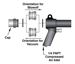
Reverse the direction of the nozzle insert to change from vacuum to blowoff.
