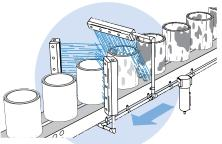
(3) Model 110012 12" (305mm) Super Air Knives blow excess honing oil off machined engine sleeves.
