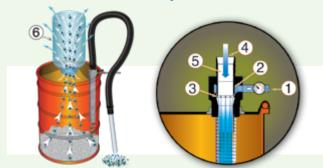
Compressed air, normally 80-100 PSIG (5.5 - 6.9 BAR), flows through the inlet (1) into an annular plenum chamber (2). It is then injected into the throat through directed nozzles (3). These jets of air create a vacuum at the intake (4) which draws material in, accelerates it through the unit (5), and directs it to the bottom of the drum. The airflow exhausts through the port in the drum lid. Airborne particles are trapped by the filter bag (6).
