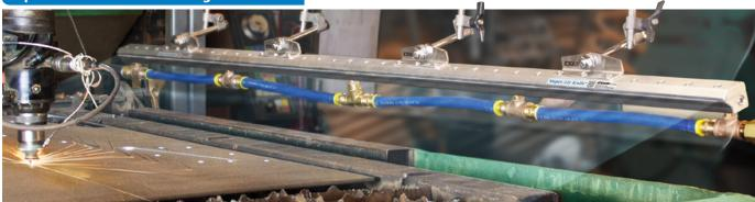
EXAIR offers Super Air Knives in lengths from 24" (610mm) through 108" (2743mm) with Plumbing Kits that are shipped fully assembled. All components have been properly sized to obtain the best performance from the Super Air Knife.
