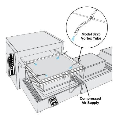
**The Problem:** A manufacturer of major appliances vacuum forms the plastic interior shell of refrigerators. The deep draw of the plastic and complex geometry left the four corners unacceptably thin. The corners would tear during assembly or bulge when insulation was inserted between the shell and exterior housing, resulting in a high rejection rate.
