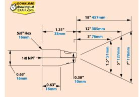
The Model HP1136SS Shim Set for the 1" High Power Flat Super Air Nozzle includes a .020" (0.51mm) and .030" (0.76mm) thick shim. A .025" (0.64mm) shim is installed
