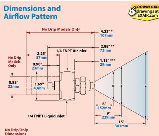
No Drip Only Dimensions in Red See page 93 for No Drip Atomizing Nozzles
