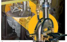
An automotive manufacturer vacuums chips from drive train differentials with a Model 150200 2" (51mm) Heavy Duty Line Vac.
