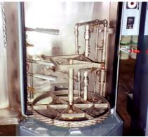
(3) Model 2012 12" (305mm) Standard Air Knives perform the drying cycle in this parts washer.
