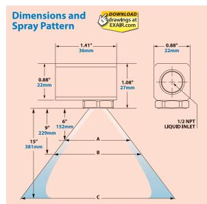
Compared to EXAIR's Air Atomizing Spray Nozzles the Hollow-Stream will have higher liquid flow rates.
