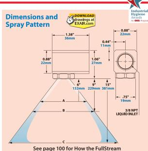
and HollowStream Cone Nozzles Work.
