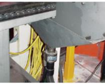
Metal parts are conveyed with the Model 150200 2" (51mm) Heavy Duty Line Vac as they drop off the edge of the conveyor.
