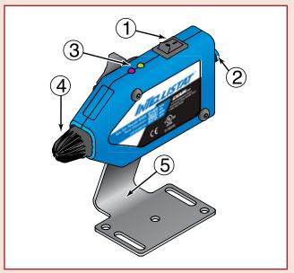
After connecting the 24V power supply, activate the power switch (1) and turn on a compressed air source to supply the 6mm push-in fitting (2) to activate the static eliminating ions and airflow. Proper or improper functionality is indicated by a green or red LED (3). The non-marring nozzle (4) provides quiet performance and OSHA compliance. The compact mounting bracket (5) is included to provide handsfree operation.
