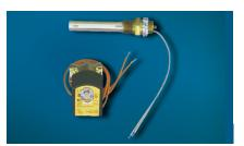
Solenoid Valve and Thermostat: Cabinet Cooler Systems with thermostat control include a solenoid valve and thermostat that limit the flow of compressed air to only cool when needed. The thermostat is factory set at 95°F (35°C). It will normally hold ±2°F (1°C) inside the cabinet. Solenoid valves are available in 120V, 60Hz; 110V, 50Hz; 240V, 50/60Hz and 24VDC. All solenoids are CSA Certified and UL Listed or Recognized.
