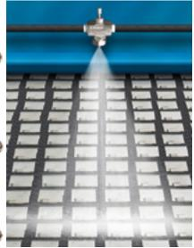
A Model AF1030SS is used to spray an anti-corrosion coating on stamped steel parts as they travel on a conveyor.
