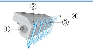
Compressed air flows through the inlet (1) into a plenum chamber. It is then throttled through a thin nozzle (2) extending the length of the Standard Air Knife. This primary airstream adheres to the Coanda profile (3), which turns it 90° and directs the flow down the face of the unit. The primary stream immediately begins to entrain surrounding air (4), for an amplification ratio of 30:1 at 6" (152mm) away.
