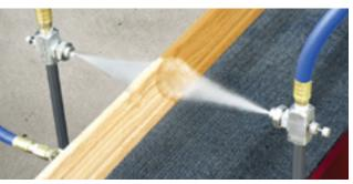
(2) Model ER1020SS atomizing nozzles are used to apply a fire retardant coating to wood trim.
