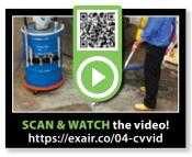
EXAIR's Chip Vac picks up dry or wet chips and delivers them directly to an ordinary open-top drum. The Chip Vac is used to clean chips from fixtures, floors and work surfaces of machining centers, lathes, saws, mills and other industrial equipment. The powerful suction is ideal for fast and efficient cleaning.
