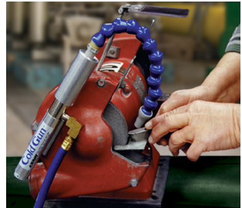
Cold air eliminates heat cracking of the carbide tool during sharpening.
