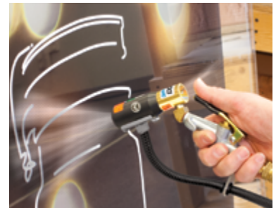
The Model 8293 Gen4 Ion Air Gun cleaning artwork and glass prior to framing.
