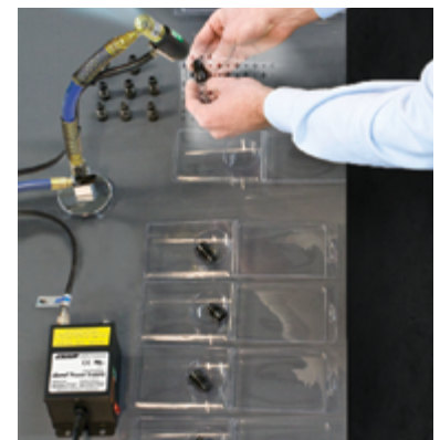
The Gen4 Model 8910 Instant Static Elimination Station removes contaminants on plastic fittings prior to packaging.
