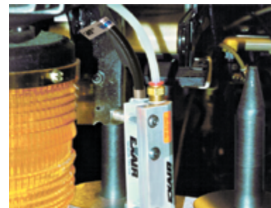
A Model 8103 3" (76mm) Gen4 Standard Ion Air Knife removes dust from computer hard disks prior to assembly.
