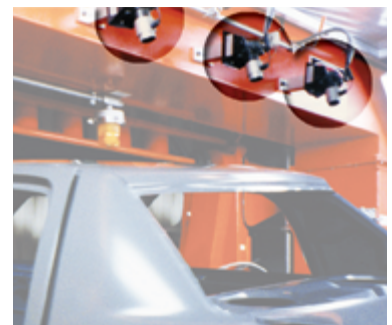
(3) Gen4 Ion Air Cannons blow contaminants from car bodies prior to painting.
