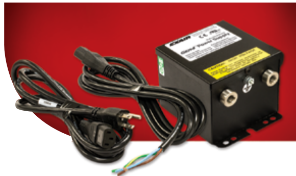
The Model 7960 Gen4 Power Supply has 115VAC or 230VAC selectable voltage, lighted power switch, integral fuse on the primary, electromagnetically shielded modular power cable and (2) 5kV outlets.
