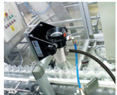
The Model 8292 Gen4 Ion Air Cannon System eliminates the static and dust prior to filling the bottles.
