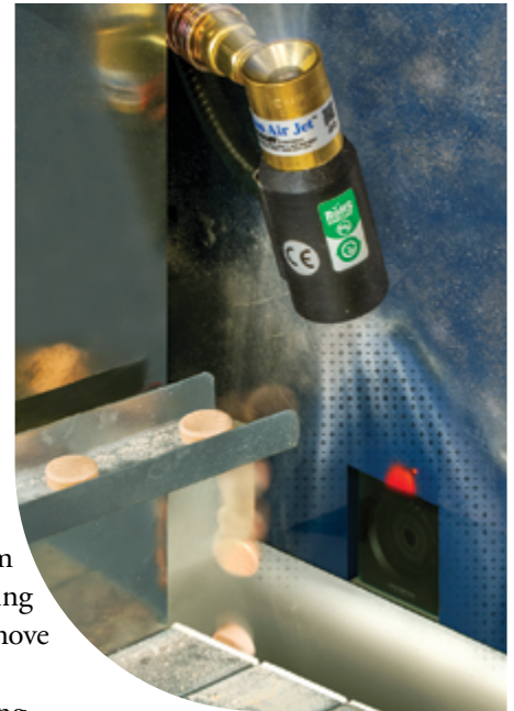
The Model 8294 Gen4 Ion Air Jet with Gen4 Power Supply neutralizes static and removes dust from a counting sensor window on a tablet production machine.
