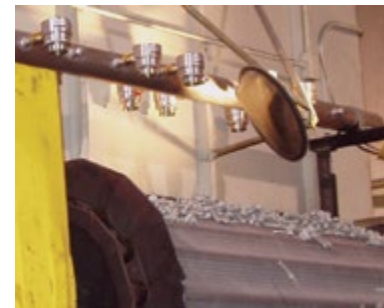
Metal parts are dried using a series of Model 6042 2" (51mm) Adjustable Air Amplifiers.
