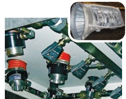
Model 120022 2" (51mm) Super Air Amplifiers and Model 1122 2" Flat Super Air Nozzles blow off transmissions after they are machined.
