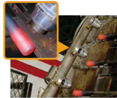
Model 6042 2" (51mm) Adjustable Air Amplifiers with swivel fittings cool inductively heated axles prior to installing the hubs.
